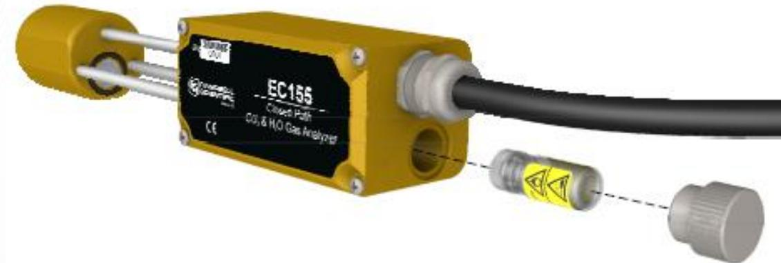
FIGURE 9-7. Replacing the source housing desiccant/scrubber bottle
