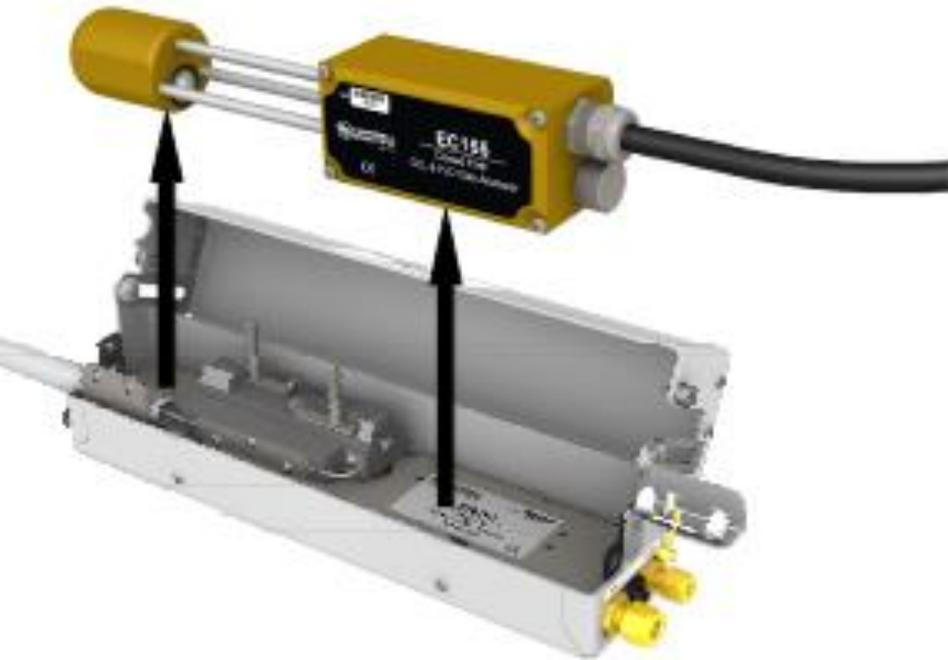
FIGURE 9-4. The EC155 analyzer and sample cell with shell top open
