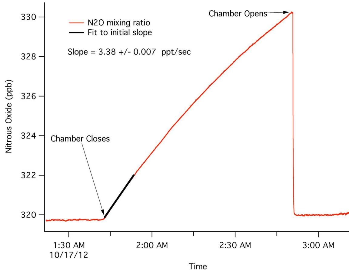
This rise rate corresponds to a small flux: 8 micro grams N<sub>2</sub>O-N /m<sup>2</sup>/hour or 0.08 nano-moles/m<sup>2</sup>/s.
